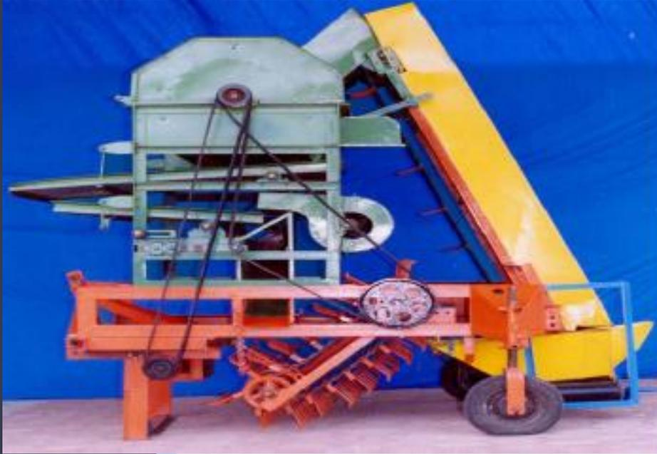
**Concave made of 6 mm mild steel rod with inner diameter of 610 mm and sieve hole size of 80 x 30 mm was provided covering the half circumferential area of cylinder.**
