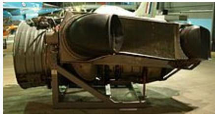
The plenum chamber burning [Bristol Siddeley BS100](#). In this [vectored thrust](#) engine reheat was applied to the front two nozzles only
