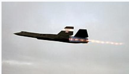
[SR-71 Blackbird](#) in flight with [J58 engines](#) on full afterburner, with numerous [shock diamonds](#) visible in the exhaust.
