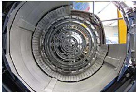
Rear part of a sectioned [Rolls-Royce Turbomeca Adour](#). The afterburner with its four combustion rings is clearly seen at the center.
