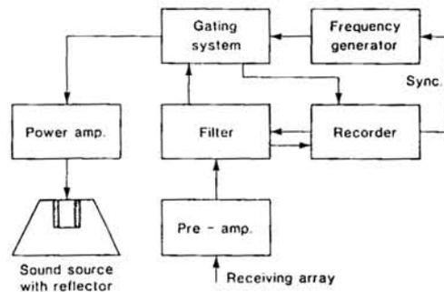
Fig. 8. Block diagram of the sonar system.
