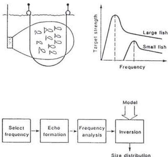
Fig. 1. Basic processes of fish length estimation by resonance echo sounding.
