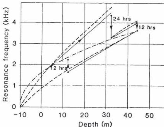
Fig. 3. Resonance frequency versus depth. --- "the law of constant gas mass" -.- "the law of constant gas volume".
