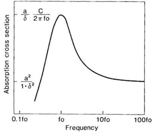
Fig. 7. Extinction cross-section.
