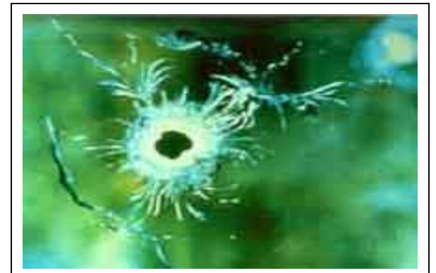
Glass fracture produced by a high-speed projectile
