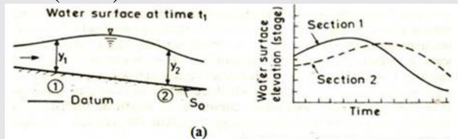
$y_1$  and  $y_2$  are the depth at section 1 and 2, respectively. In GVF, the loss of energy is essentially due to boundary friction.
