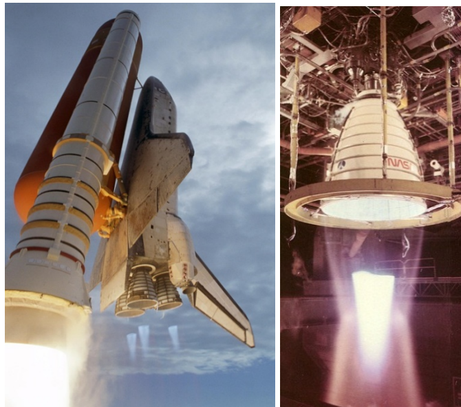
Fig. 4. Shock diamonds (blue cones) in Shuttle's main engine nozzles during STS-120 launch ( NASA ), and during tests.
