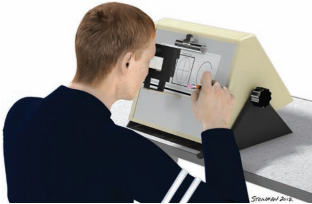
■ Figure 6.24 Keystone Correct-Eye Scope setup for cheirosopic tracing.
