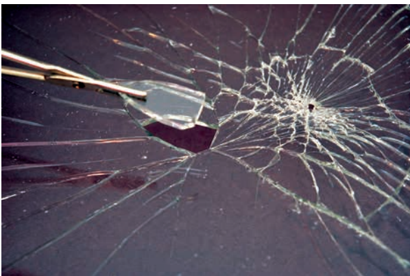
FIGURE 5-2 Matching broken pieces of glass. Finding a perfect match is tantamount to individualizing the glass to a single source with complete certainty.
