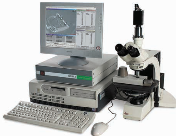
FIGURE 5-8 A hot-stage microscope is a key instrument in the forensic examination of glass. The temperature of the sample affects its density, and the density change affects the velocity of the light beam as it passes through the sample and hence its refractive index.
