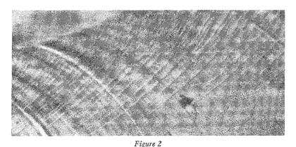
Part of chip when exactly in position showing hackle marks. Magnification ninety times.
