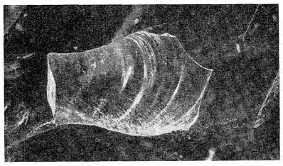
Figure 1 Chip in position on parent glass. Magnification eight times.
