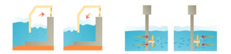
As the Earth's seas and oceans are subject to the forces and mechanisms in our solar system, large masses of water move and cause what we call the tides. The energy of this moving water can be converted into mechanical as well as electrical energy.
