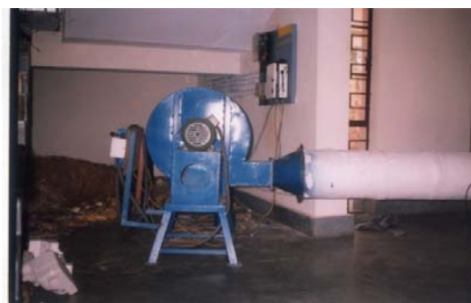
Fig. 2. Mechanical black pepper dryer
