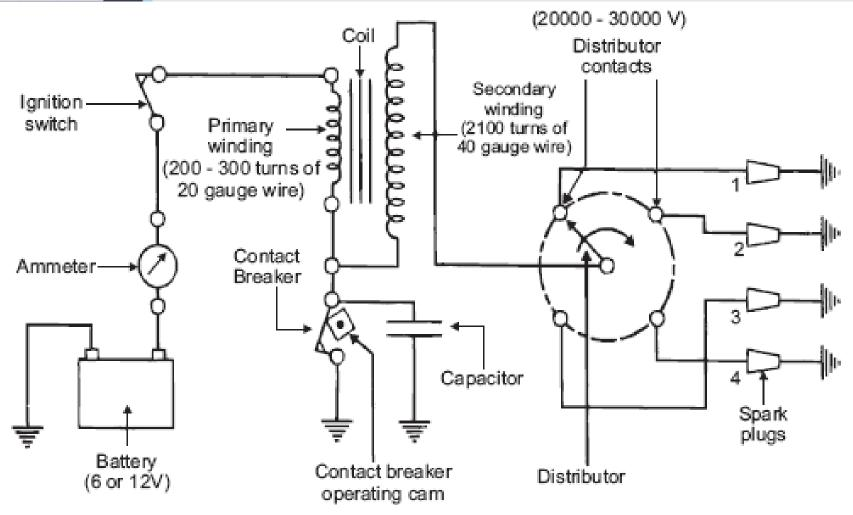
The ignition system is divided into 2-circuits :
