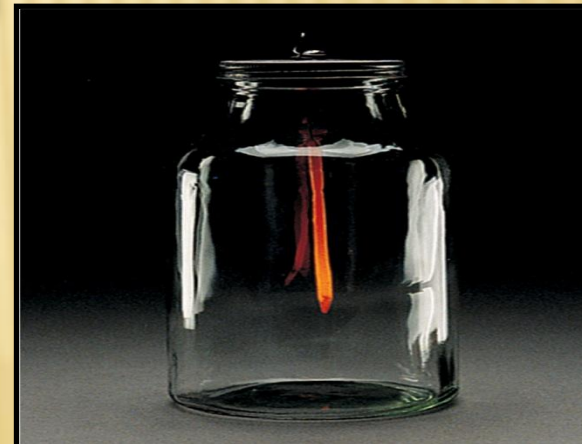
A Hot Steel nail glows feebly when placed in oxygen
