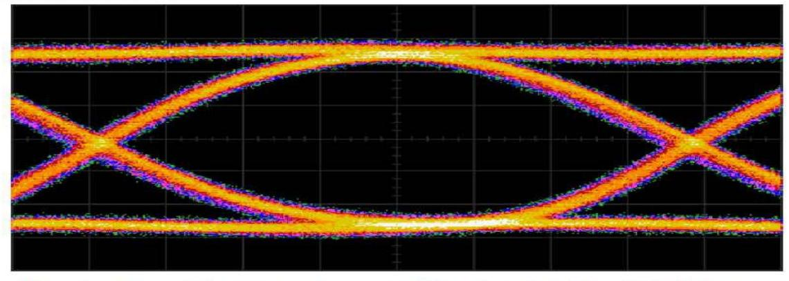
4<sup>th</sup>-order Bessel Thompson low-pass filter bandwidth = 0.75 \* bit rate
