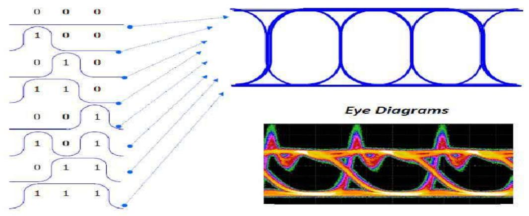
An eye diagram is a statistical representation of a bit stream, based on the contribution of randomly selected bits
