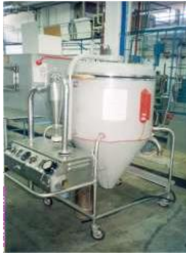
Fig. A laboratory spray dryer Main advantages of spray drying
