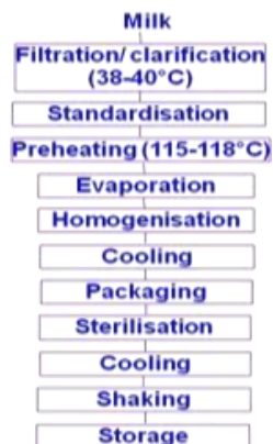
Fig. 3.11 Flow chart for preparation of evaporated milk
