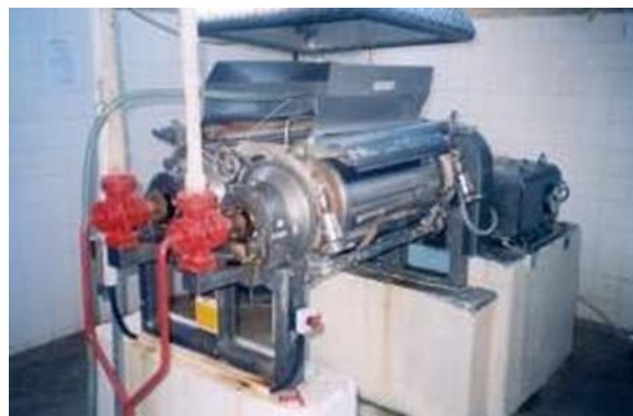
Fig. A laboratory scale double drum dryer
