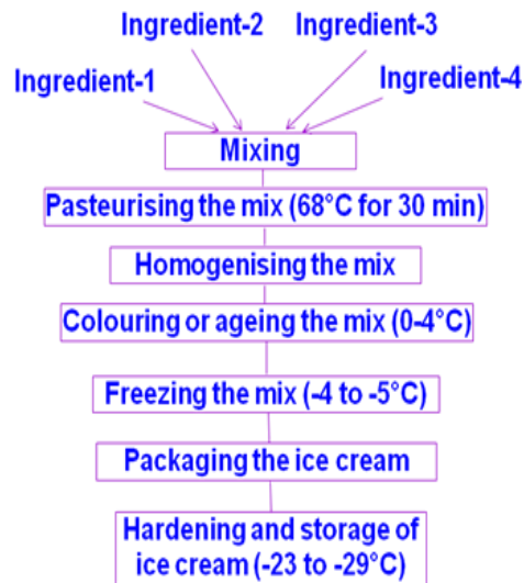
Fig. 3.7 Flow chart for preparation of ice cream
