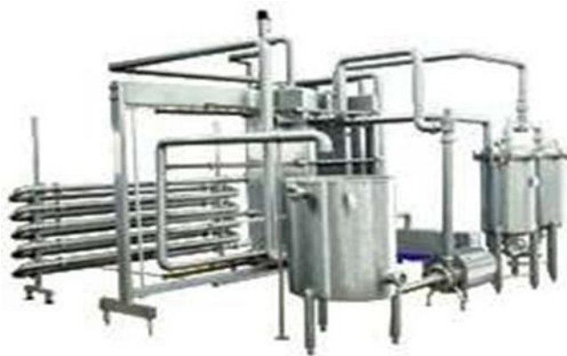
Fig. 5.7 HTST pasteurization process
