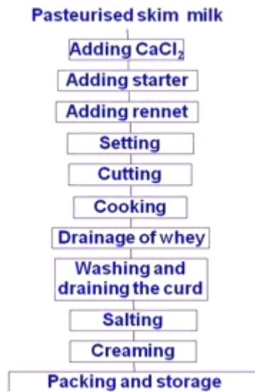
Fig. 3.9 Flow chart for preparation of cottage cheese
