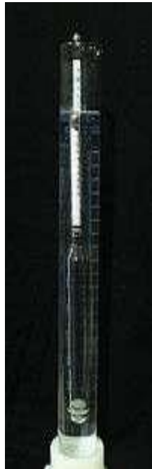
Fig. 2.2 A lactometer immersed in a cylinder
