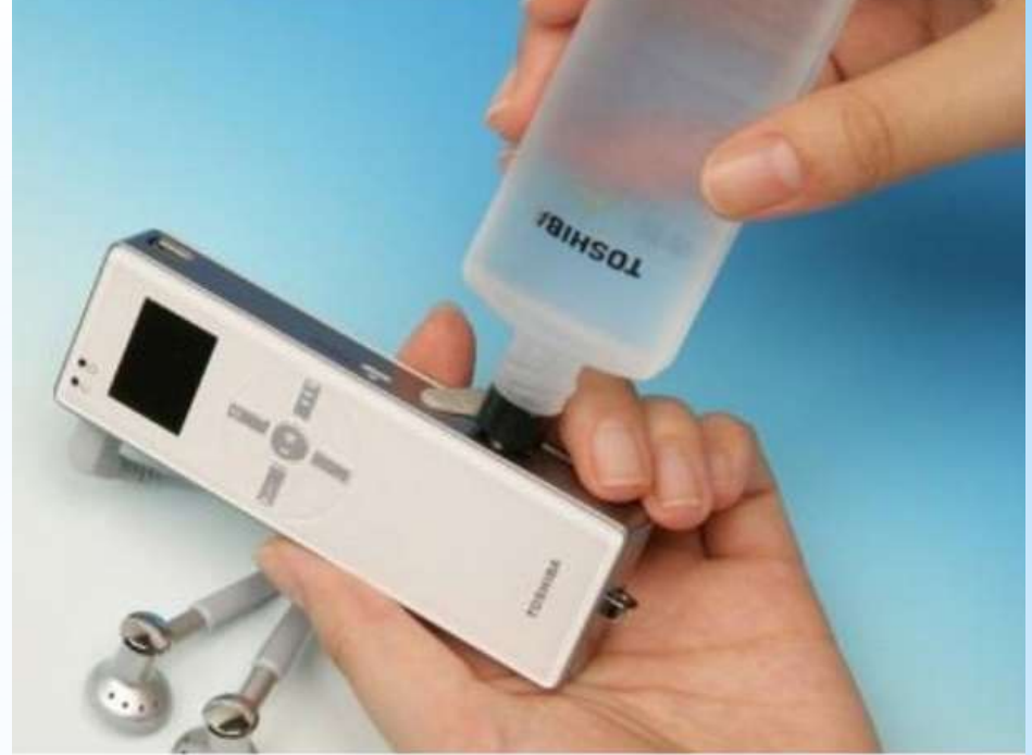
Toshiba mp3 with a fuel cell
