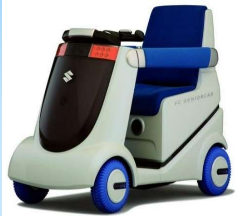
Wheel chair powered by fuel cell
