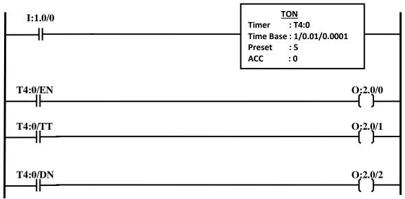
EN (Enable bit) :: This bit is high when the power to the timer block is high. i.e: 1:1.0/0 is made on. TT (Timer Time Bit) :: This bit is high when the timer is running or timer count is counting or ACC <PRE. DN (Done Bit) :: This bit is high when timer count is finished or ACC=PRE.
