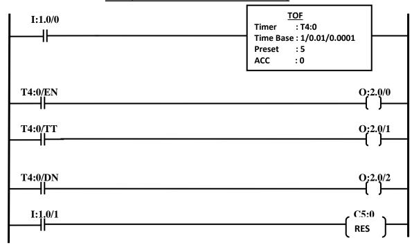
EN (Enable bit) :: This bit is high when the power to the timer block is high. i.e: I:1.0/0 is made on.
