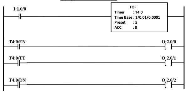
EN (Enable bit):: This bit is high when the power to the timer block is high. i.e: I:1.0/0 is made on.
