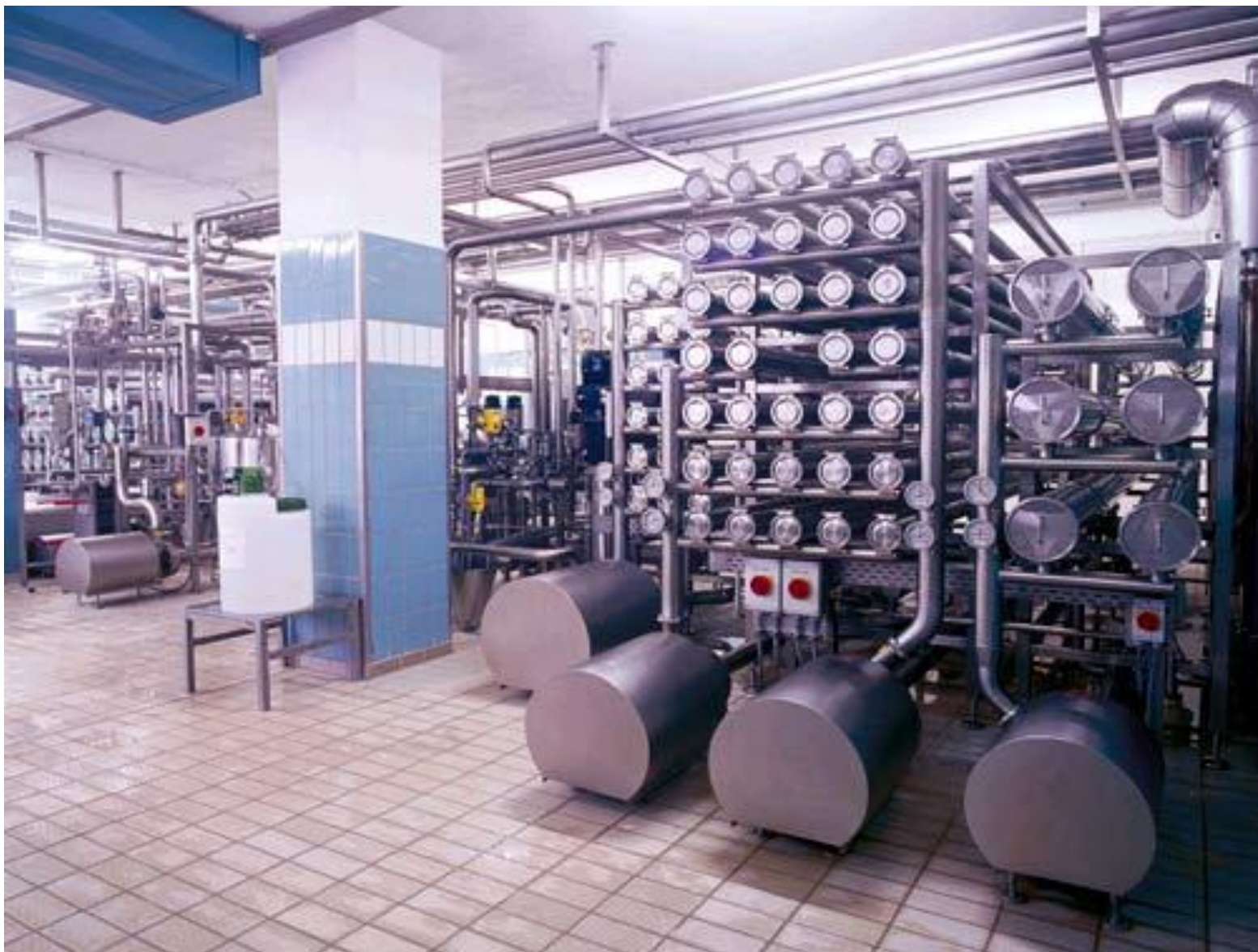
Integrated Membrane filtration system comprising UF plant for WPC & RO plant for Lactose concentration Source : DSS-Internet
