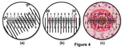
**2.** The stage micrometer is clipped to the stage and the etchings centered by moving the mechanical stage.
