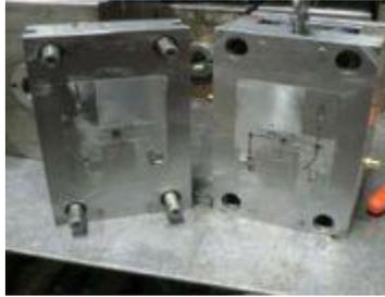
**Figure 8.1: Standard two plates tooling - core and cavity are inserts in a mold base**
