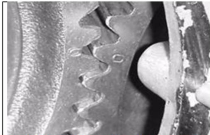
Fig: 1. View of insertion of longer end of the timing pin in the flywheel housing (Courtesy: Escort Tractor)
