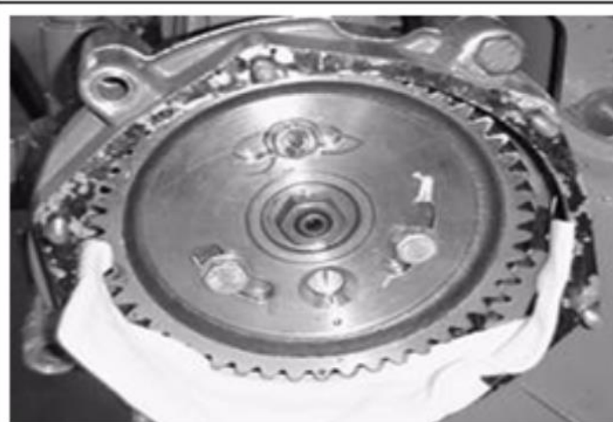
Fig: 4. View of insertion of cloth in timing inspection hole (Courtesy: Escort Tractor)
