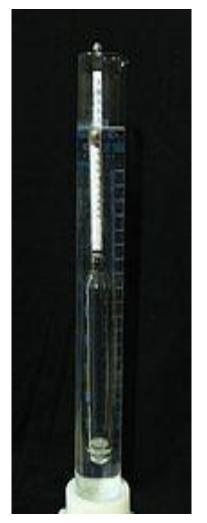
• A lactometer (or galactometer) is a hydrometer used to test milk.
