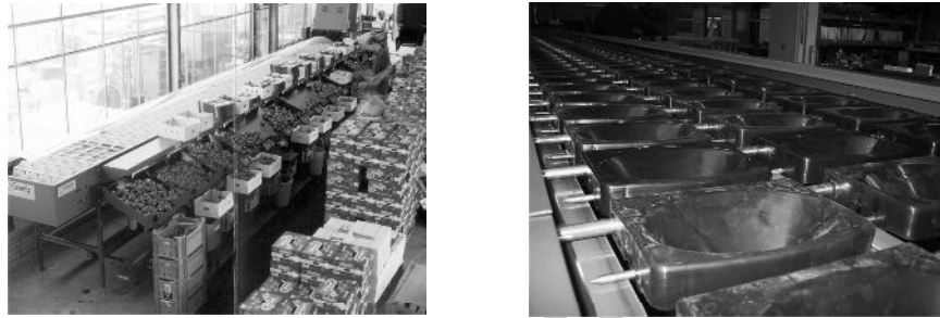
Fig. 5: Mechanical weight Grader (left), individual cups used to carry the fruit (right)
