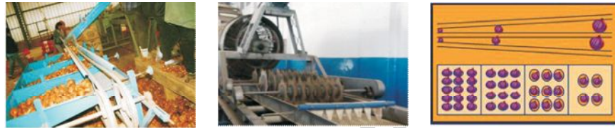
Fig. 11.8. Sizing onion bulbs by diverging belts/rope
