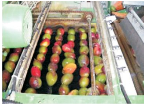
Fig. 15.1b. Wiping of wax counted commodity on coveyor.
