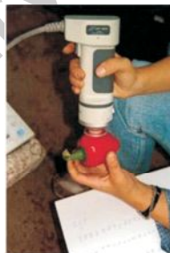
Fig. 6.2. Objective colour measurement with a colourimeter
