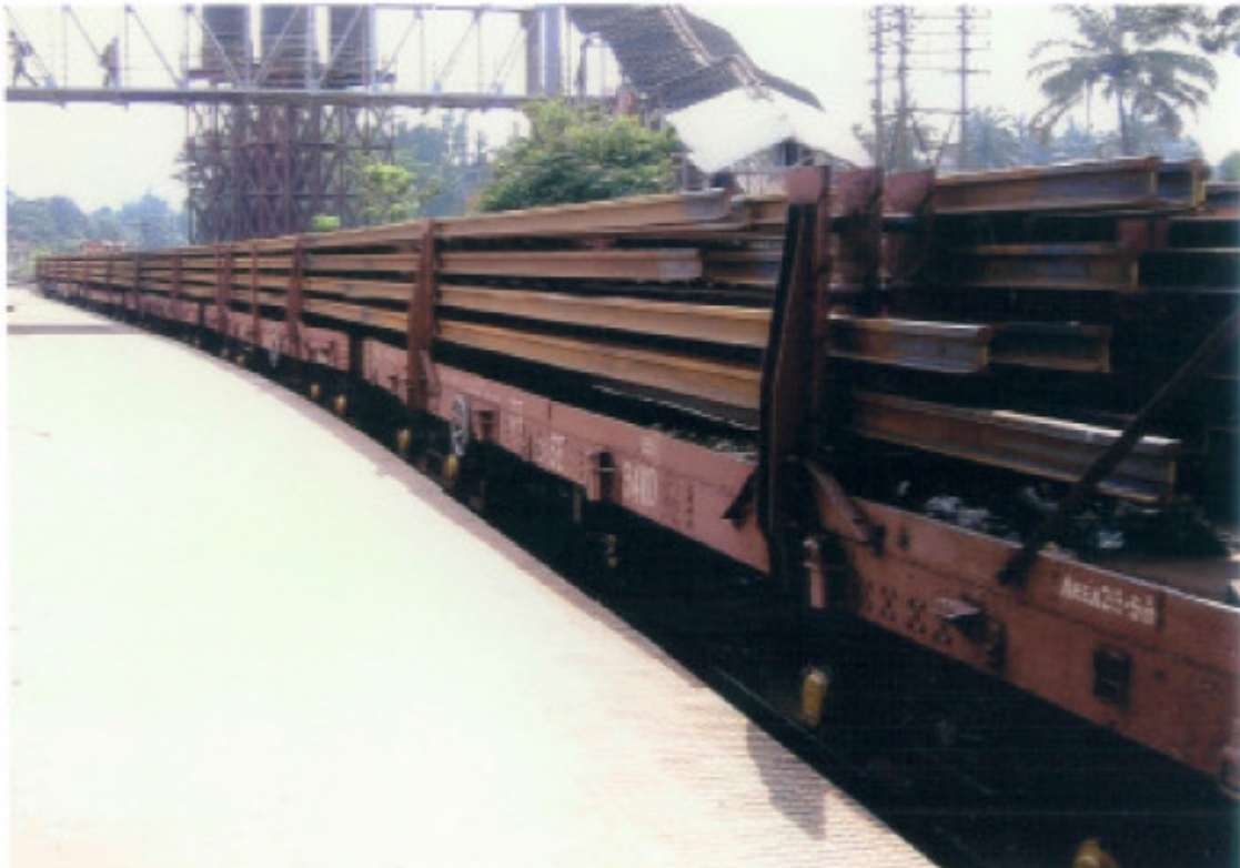
The world’s longest Rails transported on a Trailer Train-Set in India like “Spaghettis” for the Line-Doubling Programme on the Guntakal–Londa Section
