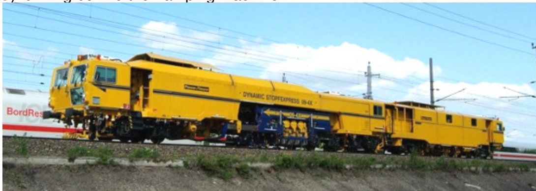
Plasser&Theurer Tamping-Express 09 cum Dynamic Track Stabiliser
