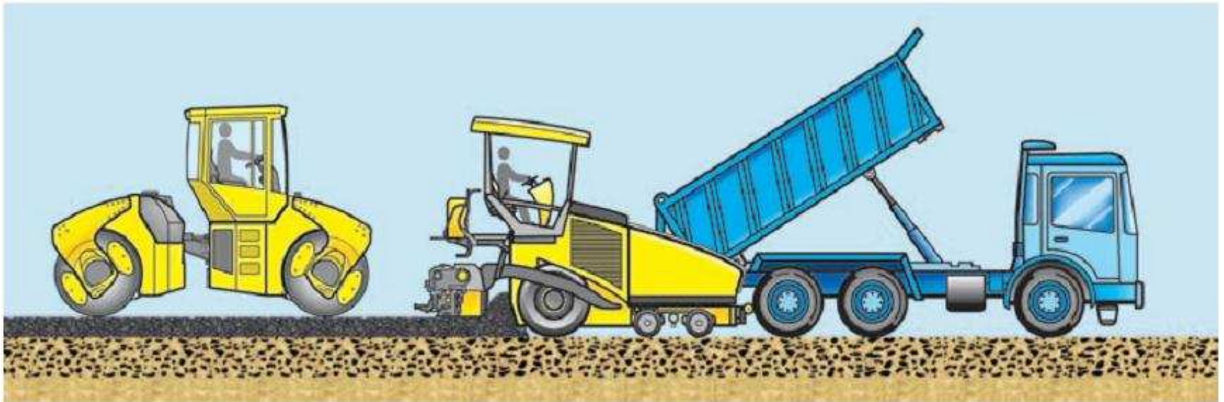
Fig. 6 Initial compaction by the finisher
