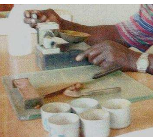
Liquid Limit test
