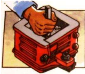
Compacting a concrete cube
