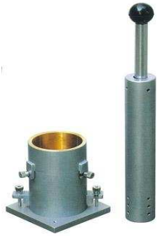
Light Compaction equipment
