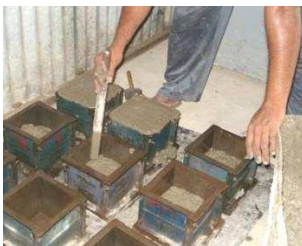
Making a set of Concrete cubes
