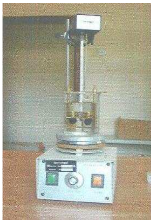
Ball and Ring Test
