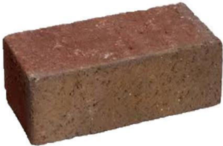
Brick = high bulk density, low pore space
