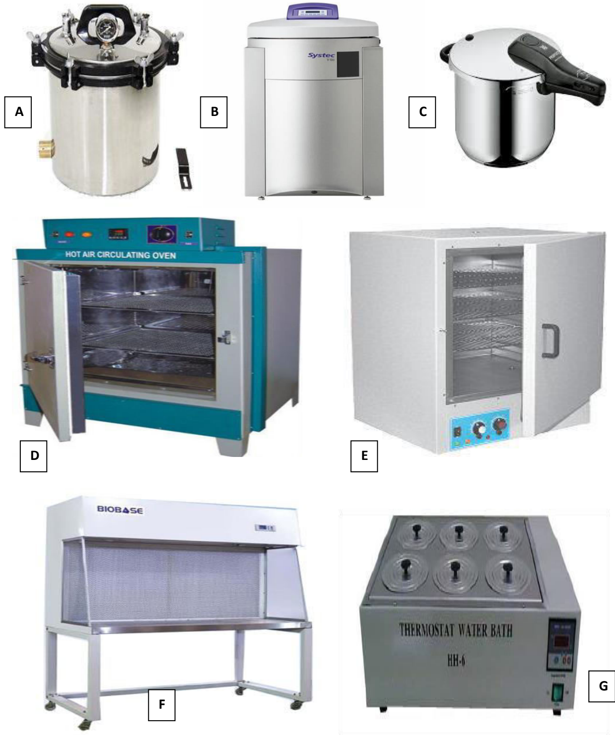
Figure 1. Manually operated (A) and automatically controlled digital (B) autoclaves, C: Pressure cooker (Stovetop autoclave), D: Oven, E: Incubator (growth chamber), F: Isolation chamber (laminar flow hood), G: Water bath
