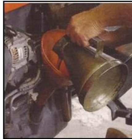
Adding oil in the engine sump
