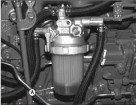
Fig: 5. View of sediment bowl (Courtesy: Escort Ltd.)
