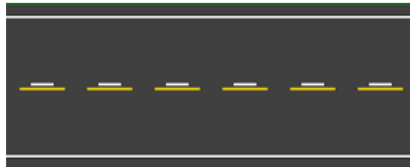
FIG.11 NO OVERTAKING ZONE LINE ON ROAD
