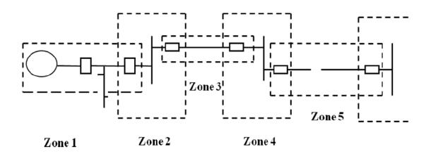
The circuit Breakers are inserted between the component of the zone and the rest of the power system. Thus, the location of the circuit breaker helps to define the boundaries of the zones of protection.
