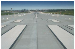
■ **Threshold Lighting** - Green lights indicate the start of the runway, and red lights indicate the end of the runway.
