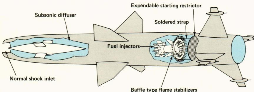
**Figure 4** — The XPM ramjet engine required a starting restrictor to permit ignition. This starting restrictor was attached within the combustion chamber with soldered straps to block the duct partially and reduce the flow velocity. On ignition, the solder melted gradually and the restrictor was blown out of the exit.
