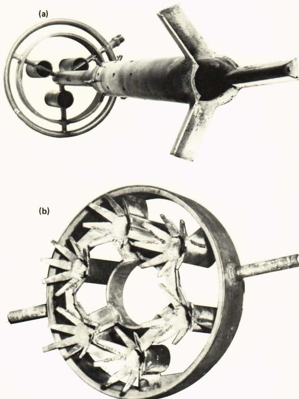
**Figure 5** — Flameholder hardware for ramjets in 1946 were combinations of blunt baffles to provide sheltered burning zones and interconnecting gutters to spread flame from sheltered piloting zones to the main fuel-air stream. View (a) shows the fuel injector and radial gutter developed for a 6-inch ramjet. View (b) shows a piloted rake for an 18-inch combustor. The central ring fits into a pilot cone and connects the pilot to the rakes by radial gutters.
