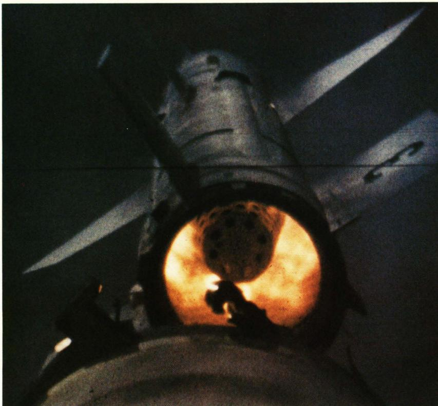
**Figure 10** — Flameholding action in the Talos combustion chamber was accomplished by vortex wakes produced by jets from holes in the central cone. Flameholding action during a Talos flight test is shown as viewed from a booster rocket.
