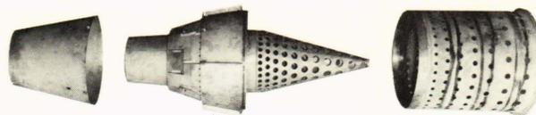
**Figure 6** — The can-type flameholder operated with good efficiency at both high and low altitudes. A fuel-air mixture flows through holes in the can wall, and recirculation zones are established behind the holes to act as flame-stabilizing elements.
