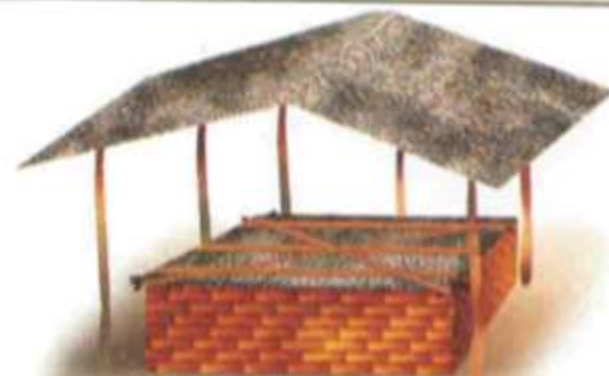
Cool Chamber under shed
