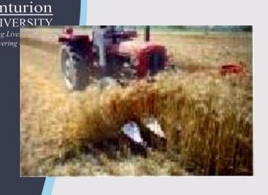
**Used for** harvesting cereal crops like wheat and paddy. It cuts the crop, conveys it vertically to one side and drops in a windrow for easy collection.
