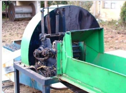
Feeding trough Feed rollers Fly wheel Cutting blade Shear plate Centurion UNIVERSITY Shaping Lives... Empowering Communities...
