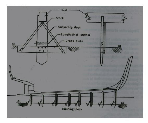
Generally good quality, hard wood timbers are used for making the building stocks. The size normally varies from 20 to 30 cms in width, 35 to 65 mm in thick and more than 1 to 2 m in length depending upon the type of boat to be constructed. Initially at one end of the stock, a slot to the size of the keel is being cut and in the other end is made to sharp to enable the builder to drive it on the ground. This type of stocks can be erected at any uneven ground with loose soil. These
