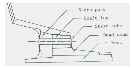
The stern tube is made up of steel in modern vessels. Brass or steel bushes are fitted on the forward and aft ends of the tube. These bushes are called stern tube bushes. The bushes are locked to the stern tube. The bushes are lined inside with soft material like lignum vitae, cutlass rubber and white metal. This complete part is called stern tube bearing. The propeller shaft or the tail end shaft rotates inside the stern tube or these stern tube bearings.
