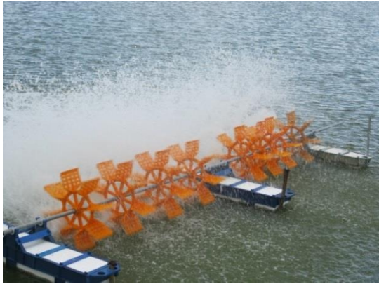
Custom made 7 wheel and 6 wheel PWA with diesel engine and modified car engine
