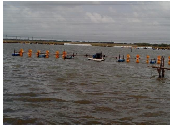
Custom made 7 wheel and 6 wheel PWA with diesel engine and modified car engine
