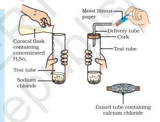
Figure 2.4 Preparation of HCl gas
