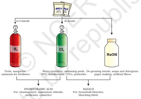
Figure 2.8 Important products from the chlor-alkali process
