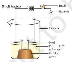
**Figure 2.3**Acid solution in water conducts electricity
