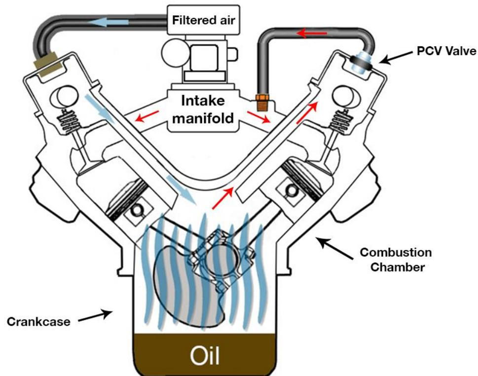
*The positive crankcase ventilation system **uses manifold vacuum to purge the crankcase blow-by fumes.** The fumes are then aspirated back into the engine where they are reburned.*
