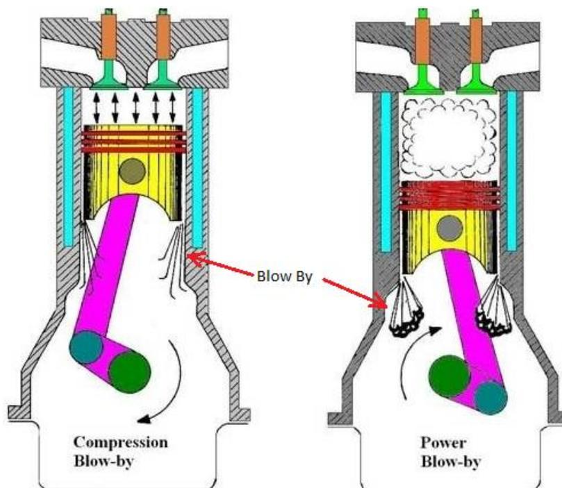
Blow by in crankcase is controlled by “Crankcase Ventilation System”. **There are two types of crankcase ventilation systems viz: -**
