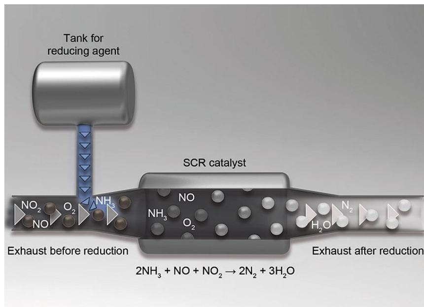
Figure above indicates the chemical reaction taking place in SCR using aqueous urea solution.
