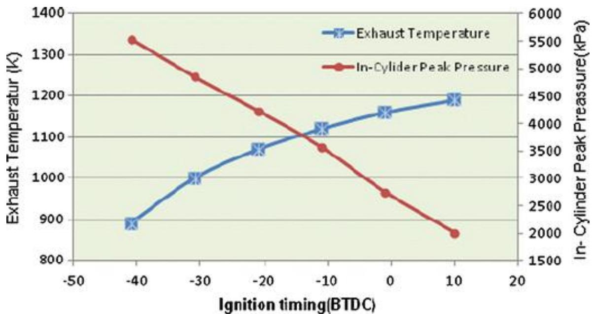
The effect of spark timing CABTDC (Crank Angle Before Top Dead Centre) on HC, NOx and CO are shown in the graphs above. Also, the effect of ignition timing on “Exhaust gas temperature” and “In-cylinder Peak Pressure” are also graphically shown.
