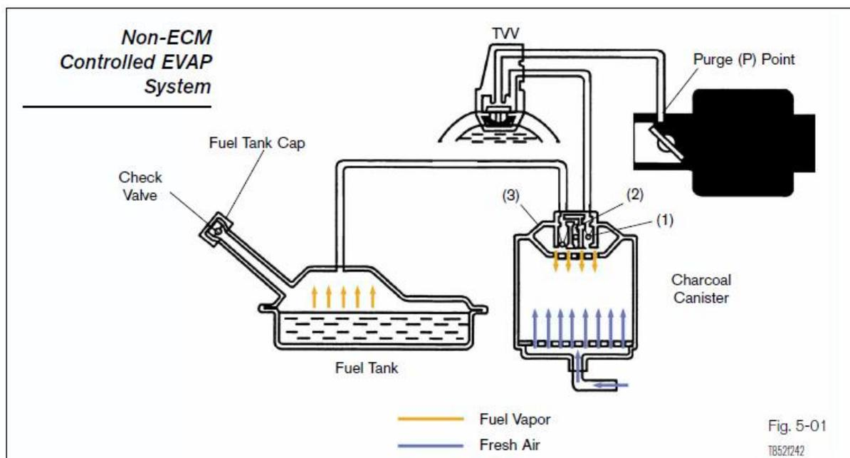
When fuel vapour pressure in the fuel tank is higher than the set value of the EVAP two-way valve (2 and 3), the valve opens and regulates the flow of fuel vapour to the evaporative emission control cannister. *Sometimes, traces of liquid vapour go along with the vapours. In that case, the vapours and liquids are separated in the fuel tank itself by a separator. The vapour goes through the separator and liquid fuel is returned to the fuel tanks.*
