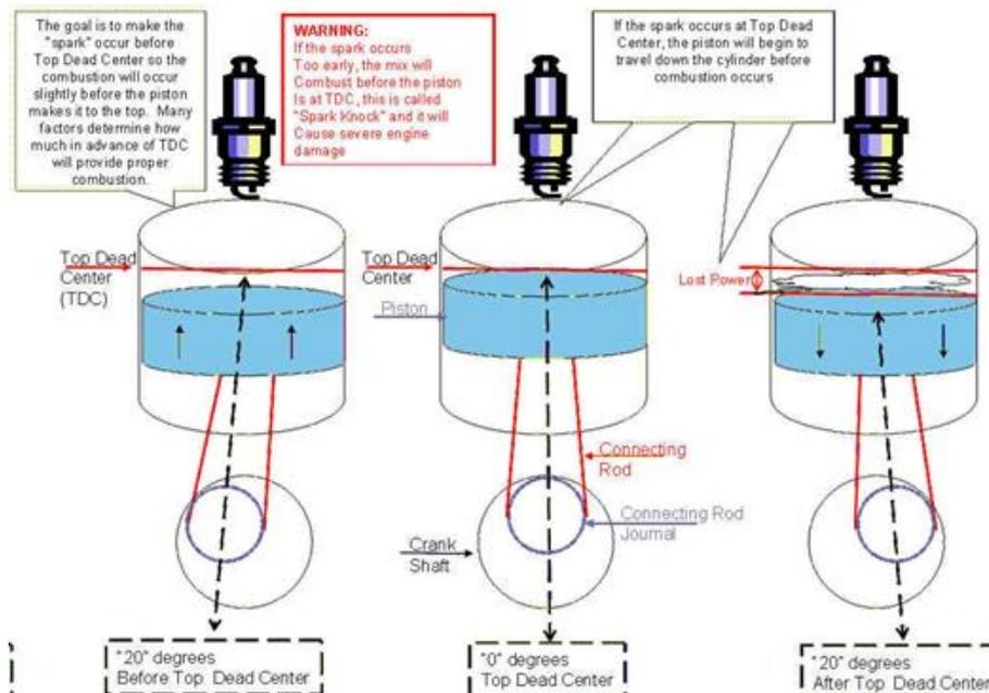
Hydrocarbon emission decreases with increased spark advance. The better combustion at advanced timing effects in reduction of the hydrocarbon emission.
