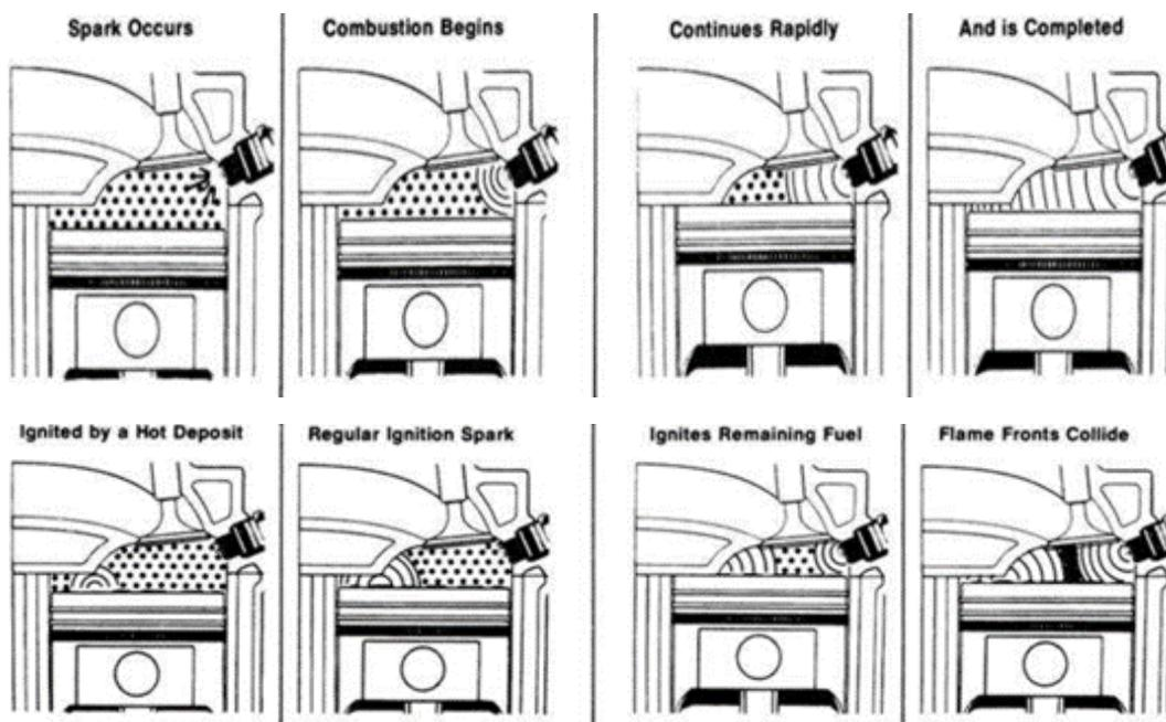
Note: It takes some time for the air and fuel mix to combust after the Spark Plug “Sparks”
