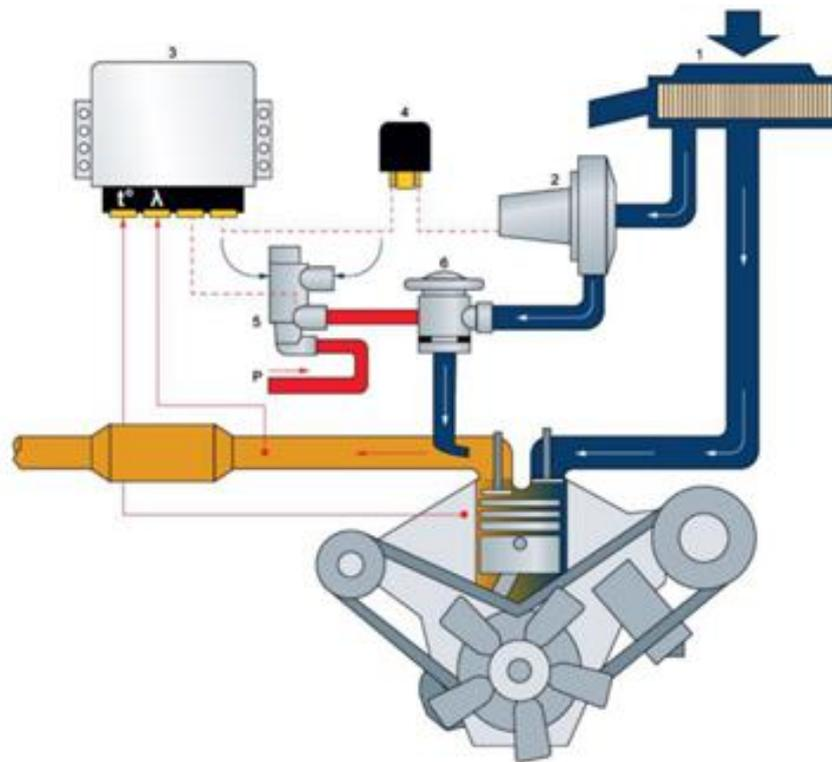
1. Air filter 2. Secondary air pump 3. ECU 4. Control relay 5. Change-over valve 6. Combination valve
