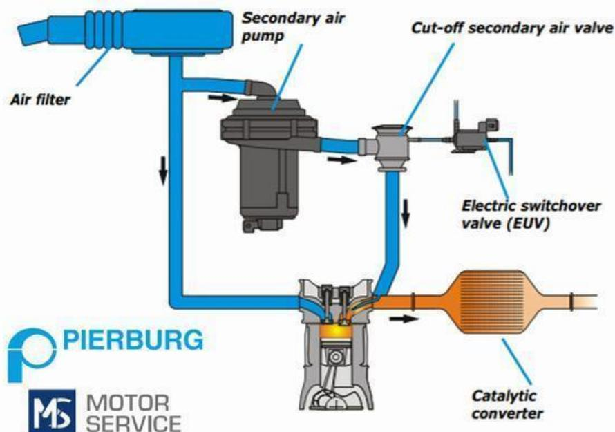
In this system, *the air injection pump (driven electrically in modern cars) blows fresh air into the exhaust stream under certain operating conditions. The air is blown through the air lines and air manifold into a series of air injection tubes which are located opposite to the exhaust valves. The oxygen in the air helps in burning of the unburnt fuel particles present in the exhaust manifold.*
