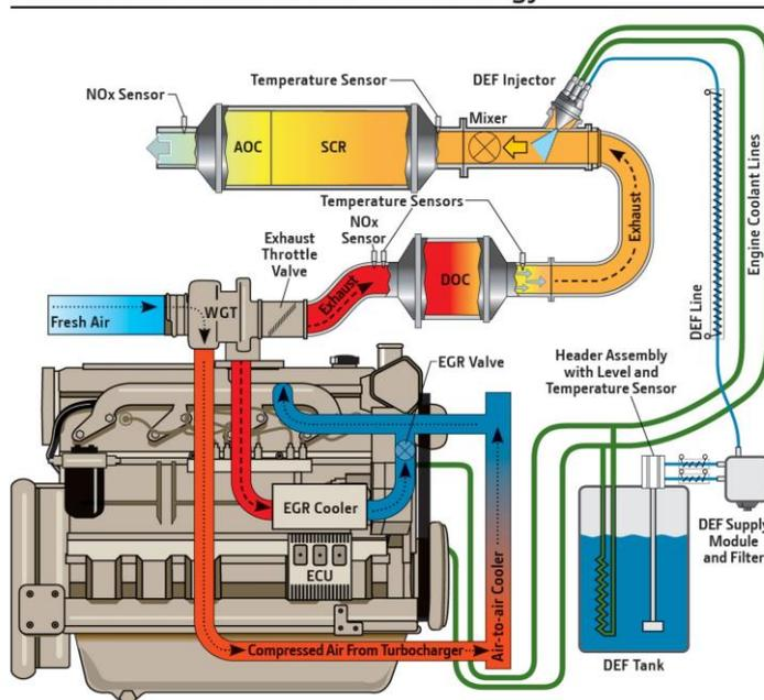
Picture below shows a MAN (Euro-VI) Truck Diesel Engine with 2-Stage Turbocharging using combined EGR and SCR technologies with Oxidation catalyst and DPF for exhaust emission
