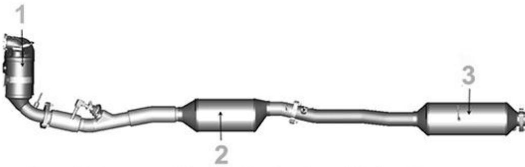
Figure 1: Common Exhaust Aftertreatment System Sequence
