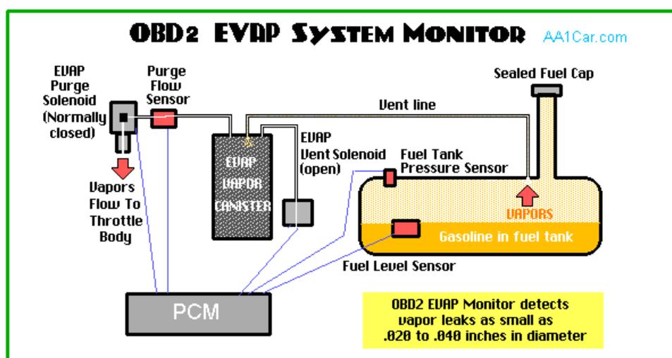
When the engine has reached predetermined parameters (closed loop, engine temp. above 52°C, stored fuel vapours are purged from the canister whenever the purge VSV is opened by the ECM. At the appropriate time, the ECM will turn on the purge VSV. This will allow the low pressure in the intake manifold to draw the fuel vapours out of the charcoal canister. The vapours will then be burned in the combustion chamber.
