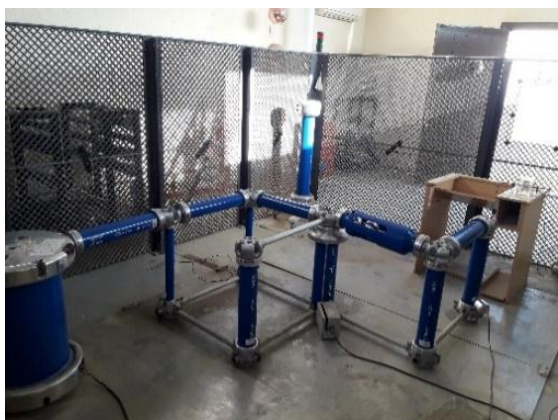
Figure 1. Experimental setup for generation the impulse voltage
