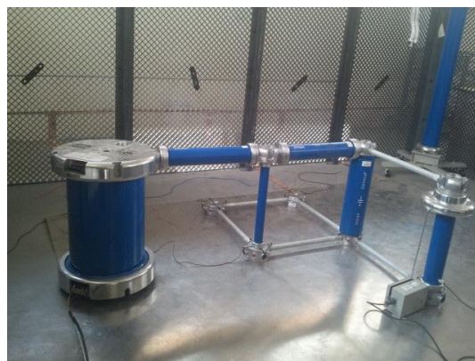
Figure 3. Experimental setup for generation DC high voltage
