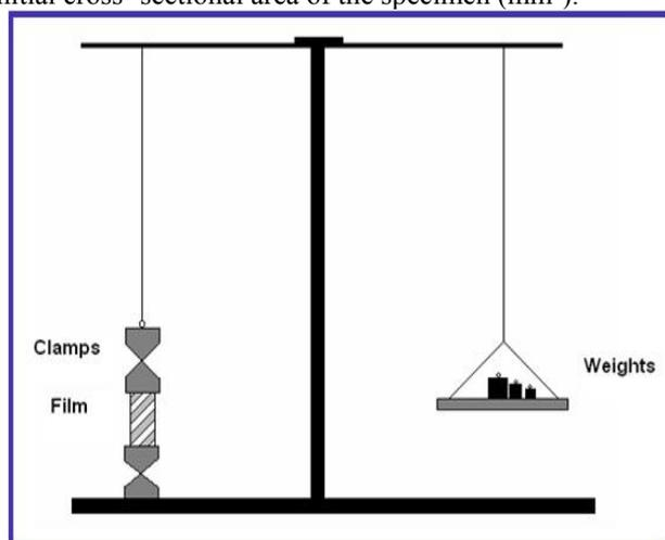
**Modified tensile strength tester.**
