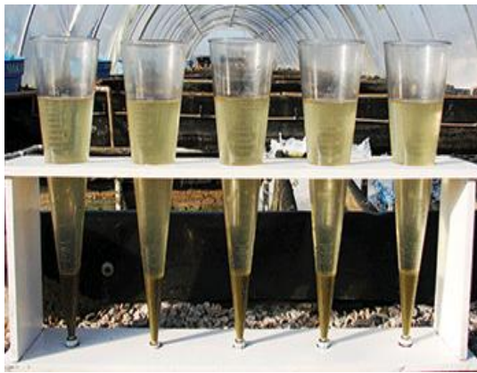
Biofloc collecting device
