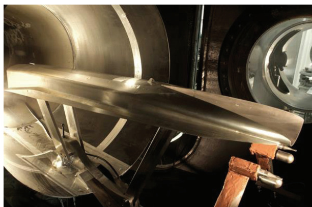
Figure 45 - View of the SSFE model installed in the F4 test section
