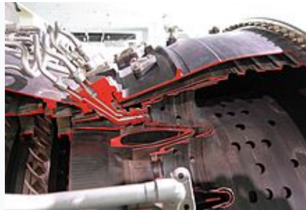
Fuel injectors of a swirl-can combustor on a Pratt & Whitney JT9D turbofan
