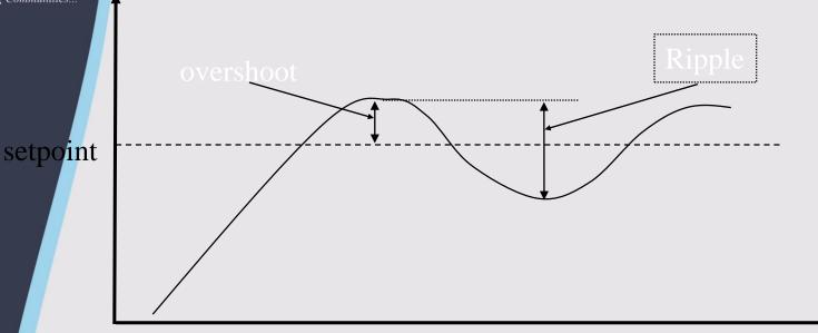
Increase the quantity until you get to the setpoint Temperature, angle, speed, etc
